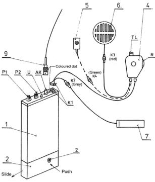
Configuration for covert operation. The lapel microphone (5) was probably not always issued. The cable to the separate PTT unit (4) was usually led through a sleeve of the coat allowing operation of the PTT button and volume control.
